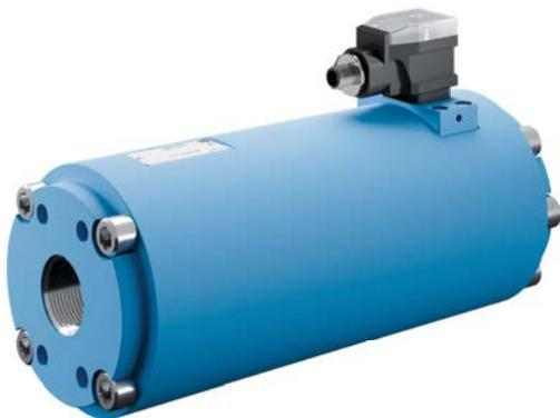
SVC flow meters with IO-Link technology are based on standard SVCs with two sensors. Unlike the versions with pre-amplifier which always send a square-wave signal to the electronics, IO-Link devices have the added capability of internally computing concrete measurement values. Therefore, these flow meters lend themselves for use in classic PLC and in IO-Link infrastructures.
