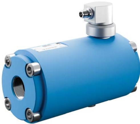
Compared with standard sensors, encoders are capable of generating considerably more pulses, thus increasing measurement resolution by orders of magnitude. Encoder-equipped SVC flow meters generate up to 2 500 pulses per revolution and can recognise the direction of flow.
