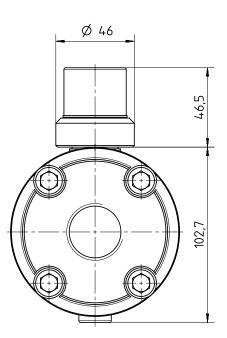
SAE connection (Code 61), maximal sensor resolution
