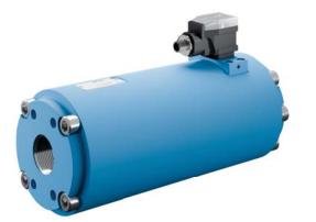
SVC flow meters with IO-Link technology are based on standard SVCs with two sensors. Unlike the versions with pre-amplifier which always send a square-wave signal to the electronics, IO-Link devices have the added capability of internally computing concrete measurement values. Therefore, these flow meters lend themselves for use in classic PLC and in IO-Link infrastructures.
